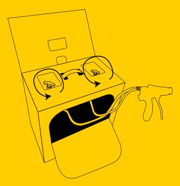
3. Open valves. Top flap may be removed or left in place during use or storage. Extend attached gun hose assembly.
