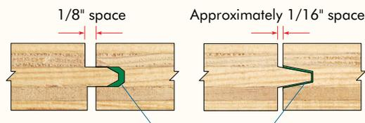
In Glued Floor Systems, use adhesives conforming with AFG-01 or ASTM D3498.
