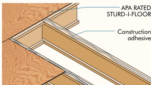
**Step 4: Nail panels correctly to prevent squeaks.** The correct nail size and spacing for your job depends on your joist spacing and panel thickness, as well as the type of panel product you are using. Attachment schedules and fastener recommendations are provided in Table 1.
